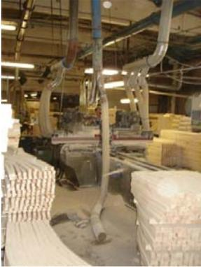
machining should be completed before wood is brought on to site. Once on site, safe work methods and local exhaust ventilation on power tools should be used. Where all other methods are inappropriate, personal protective equipment should be provided. Disposable masks must be suitable and need be changed regularly. Exposures to dust from manufactured boards, medium density fibreboard (MDF), chipboards and plywood can present additional risks when machined. Dusts can be very fine and the dust is
