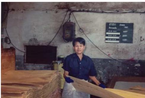
Pesticides are used to treat timber to prevent insect or fungal infestation. Many contain metals like copper, chromium and arsenic (CCA), sometimes this is visible in sunlight as a slight green colour on the timber. Other pesticides used to treat timber can also cause cancer, for example, lindane,
